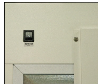
Figure 5: Defrost Cycle Switch – Top left side on the back of the incubator
